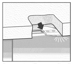
The left side of the reflector and the optic indicator in the the control panel must line up for the reflector to work.
